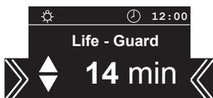
After the „Life - Guard“ - time has expired, the sauna heater is switched off and the set „Life - Guard“ - time blinks.
