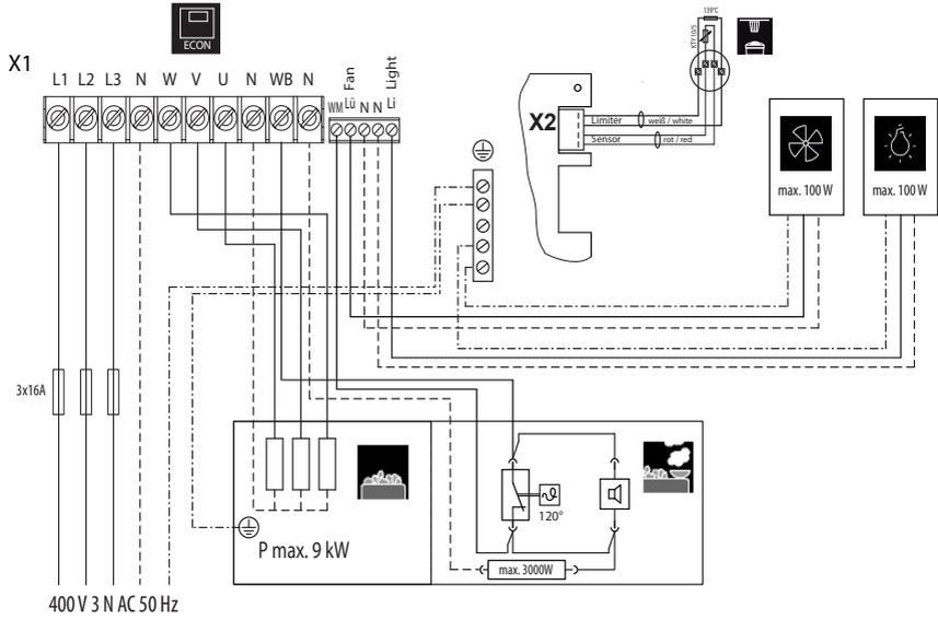
**⚠ Caution:** Always connect the neutral conductor (N) of the sauna stove. In humidity mode, one phase of the sauna stove is deactivated, i.e. the heating load is not symmetrical. The result is that the neutral conductor is then no longer currentless.
