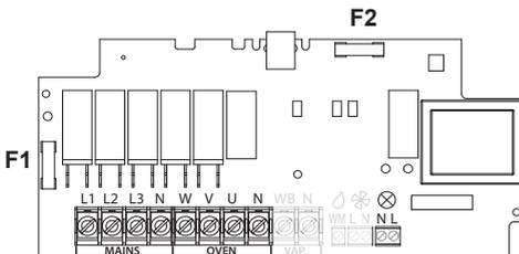
\*) specific layout of the board and its components may vary slightly from model to model.
