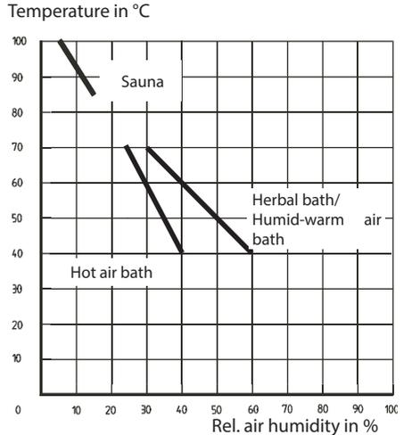
The humidity intensity shown in the display corresponds to the time-proportional vaporizer setting. Therefore the relative air humidity is not pre-selected or shown in the display, instead the activation frequency of the vaporizer is shown as a percentage. This is explained in the diagram.
