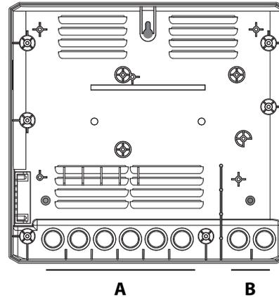
**A** Lines with mains voltage, e.g. mains supply line, heat
