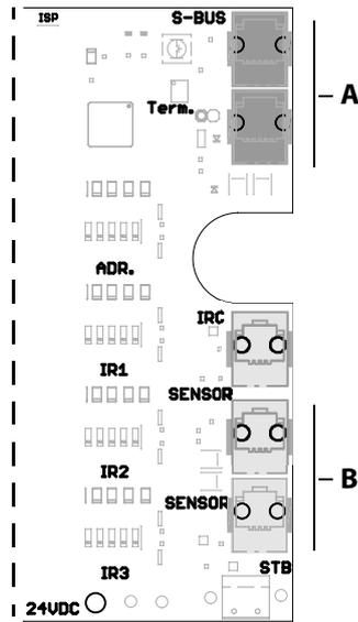
**A** RJ14 plug from control unit    **B** RJ10 plug for sensor line
