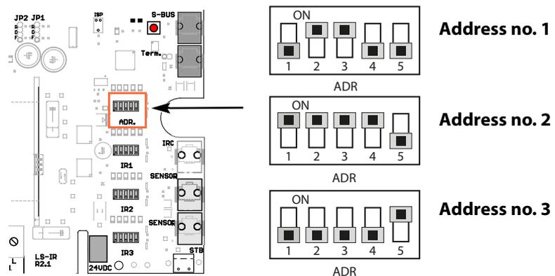
① The module is set to address no. 1 by default. This setting must be changed depending on the cabin type:
