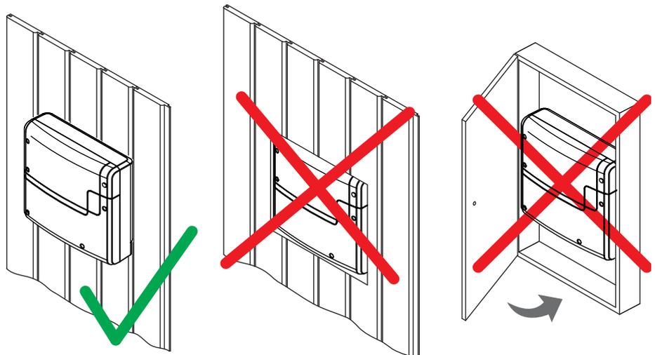
☒ Proper and improper module installation
