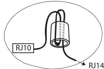
The ferrite ring for jack #1 is included in the scope of delivery for each control unit and add-on module.
